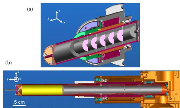
**Fig. 2.** Scheme of the aerodynamic lens system of SPLAM and its *z*-translation mechanism (vertical cuts). **(a)** View of the five lens orifices and the relaxation chamber. **(b)** View of the ALS integrated into the first two pumping stage regions (drawings: Mecaconcept).
