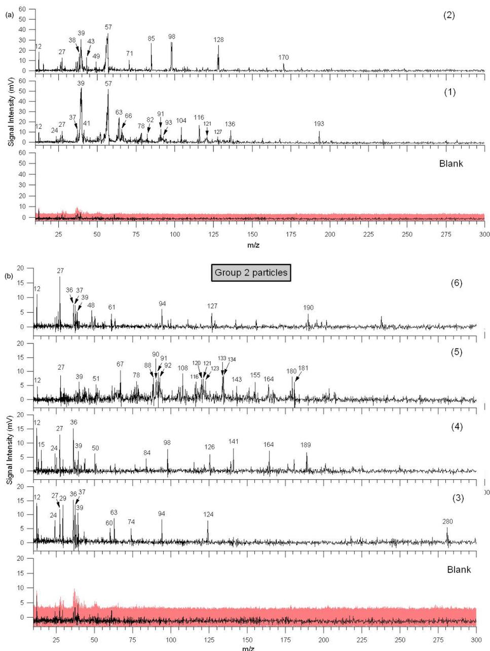
**Fig. 10.** Six single particle mass spectra of SOA produced by ozonolysis of indene in the smog chamber CESAM (group 2 particles). (a) and (b) have different ordinate scaling. The blank level is determined to be at 4 mV (indicated as red shaded zone in the lowest panels). See text for further explanations.
