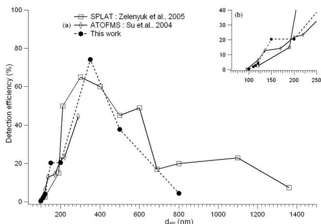
**Fig. 5.** (a) DOP particles detection efficiency for SPLAM instrument (black circles) and PSL particles detection efficiency for SPLAT (Zelenyuk et al., 2005) (open squares) and ATOFMS (Su et al., 2004) (open diamond) instruments plotted as a function of vacuum aerodynamic diameter, (b) close up of the graph (a) between 50 and 250 nm.
