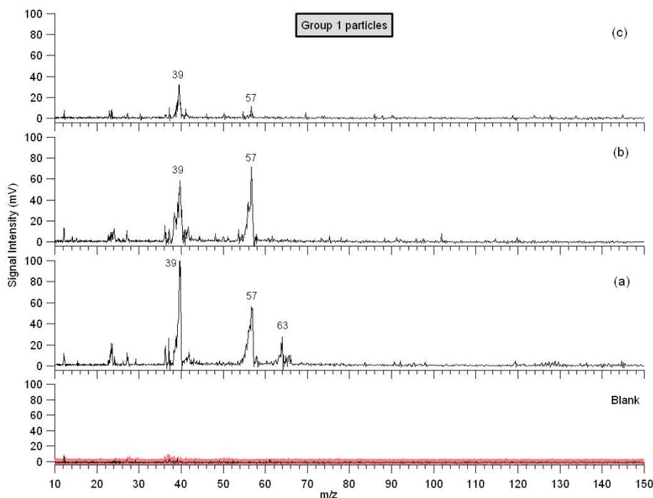
**Fig. 9.** Blank: typical noise level on the mass spectra obtained for a single laser pulse (SPLAM inlet open, CESAM chamber filled with synthetic air and ozone but without indene). The blank level is determined to be at 4 mV (indicated as red shaded zone). See text for further explanations; (a), (b), (c): examples of three single particle mass spectra of SOA produced by ozonolysis of indene in the smog chamber CESAM (group 1 particles).
