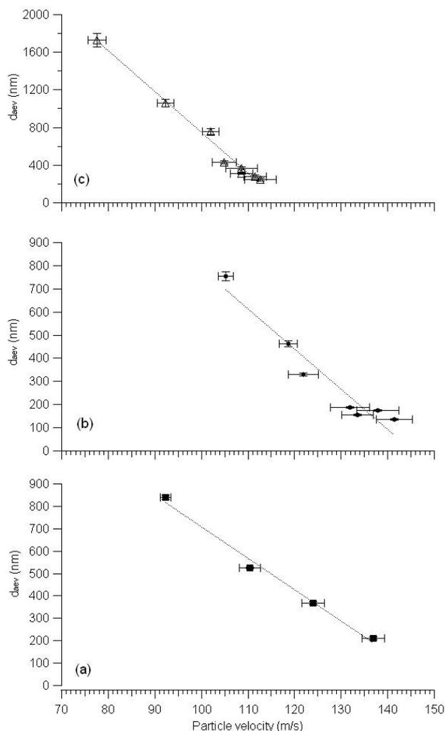
**Fig. 4.** Experimental calibration curves for aerodynamic particle sizing of the SPLAM instrument obtained for (a) – PSL, (b) – DOP and (c) – NaCl particles. The dash lines correspond to linear guideline.
