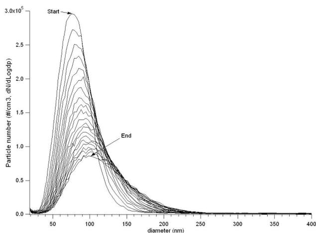
**Fig. 8.** Temporal evolution of the size distribution of produced SOA. Between the beginning and the end of this experiment, the mean diameter of the measured size distribution was shifted from 80 to 100 nm with maximum number concentrations of  $4 \times 10^3$  to  $1 \times 10^3$  particles cm<sup>-3</sup> respectively.
