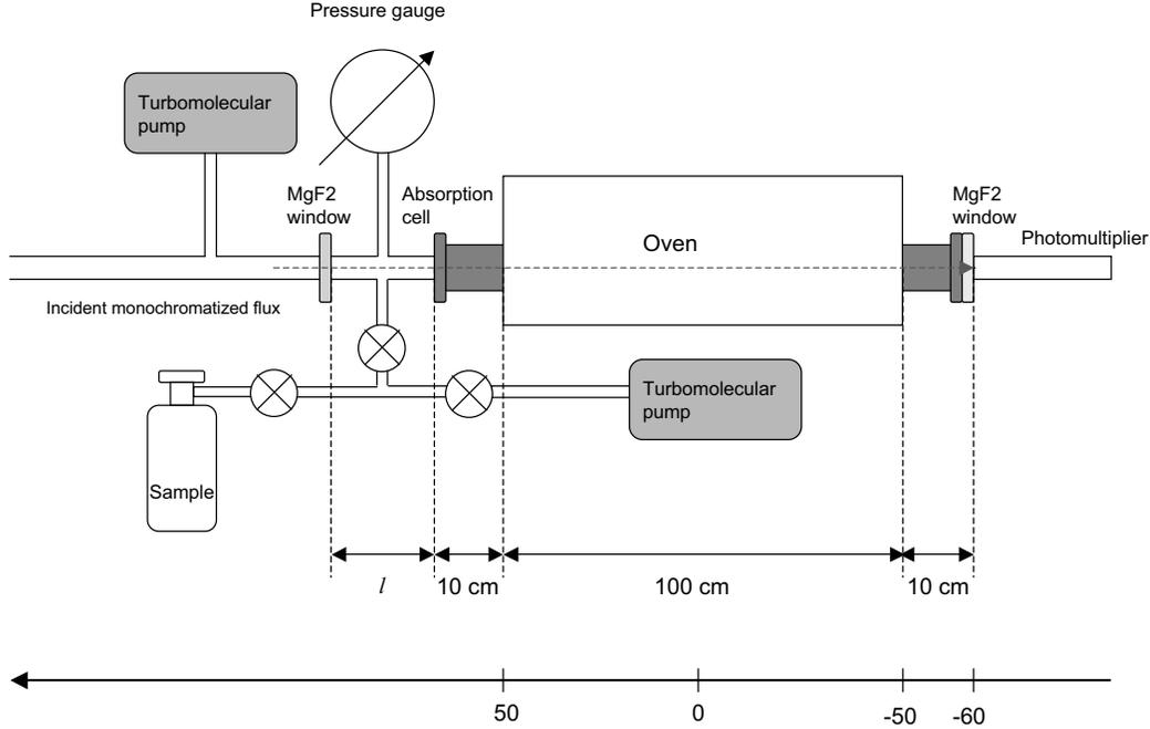
Fig. 1: Experimental setup used for measuring the ultraviolet absorption spectra at high temperatures. The length  $l$  changed during the different set of measurements. For the 115–200 nm experiments,  $l = 13.3$  cm. For the 195–230 nm range,  $l = 27.0$  cm. Finally, for the temperature calibration,  $l = 20$  cm.
