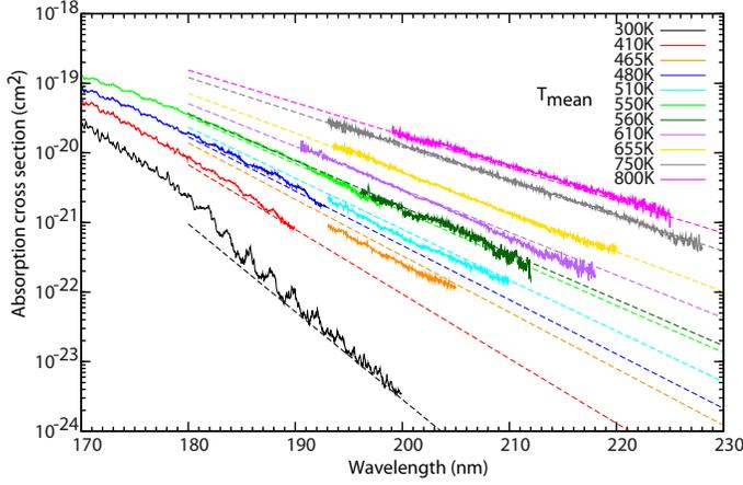
Fig. 8: Absorption cross section of CO<sub>2</sub> for wavelengths longer than 195 nm at 465 K, 510 K, 560 K, 610 K, 655 K, 750 K, and 800 K, plotted with the cross section at ambient temperature (black) and the absorption cross sections measured at shorter wavelengths and presented in Fig. 7 (300 K, 410 K, 480 K, and 550 K). The absorption cross sections calculated with Eq. 6 are plotted with the same color coding.
