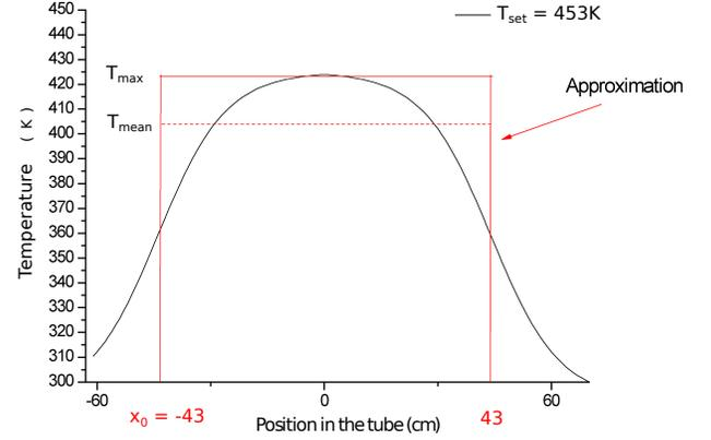
Fig. 5: Temperature inside the absorption cell for  $T_{set} = 453$  K. The maximum temperature  $T_{max}$  is 420 K and the mean temperature  $T_{mean}$  is  $(410 \pm 15)$  K. The portion of gas out of the range  $[-x_0; x_0]$  is considered at ambient temperature.
