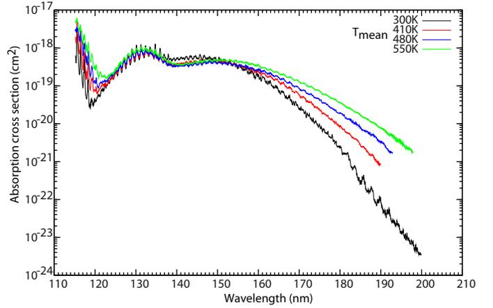
Fig. 7: Absorption cross section of CO<sub>2</sub> at  $T_{\text{mean}} = 300 \text{ K}$  (black), 410 K (red), 480 K (green) and 550 K (blue) for wavelengths between 115 and 200 nm.
