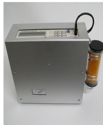
Complete system closed, with attached dryer
