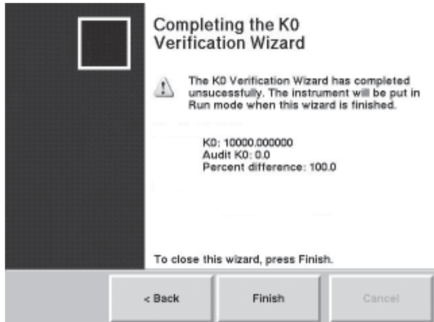
Figure 5-87. Completing the K0 Verification Wizard screen with a fail message.
