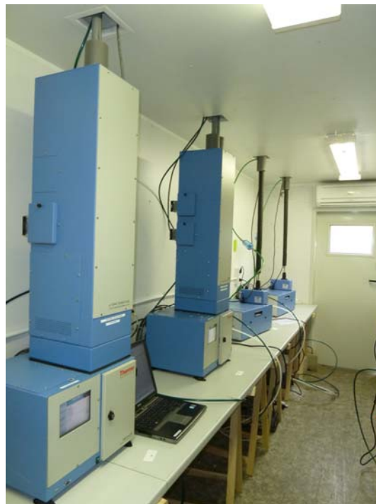
Figure 6: Measuring device TEOM 1405-F Ambient Particulate Monitor (1 st system from left) in measuring station
