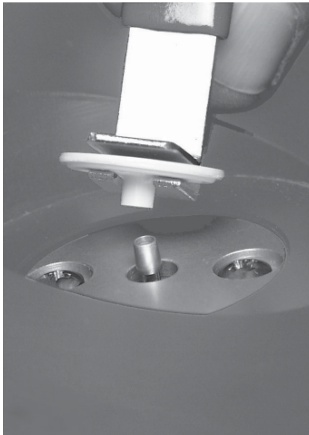
Figure 5-8. Placing the filter on the tapered element.
