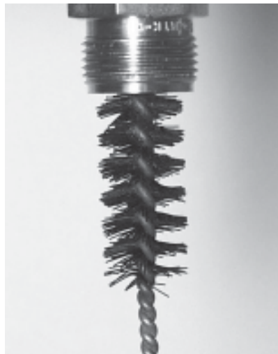
Figure 5-46. Cleaning the valve with the valve brush.
