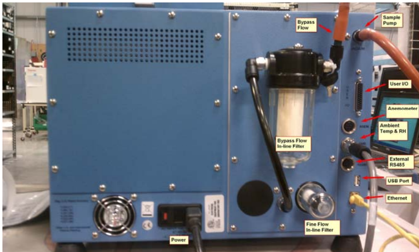
Figure 28: View on rear of the device TEOM 1405-F Ambient Particulate Monitor
