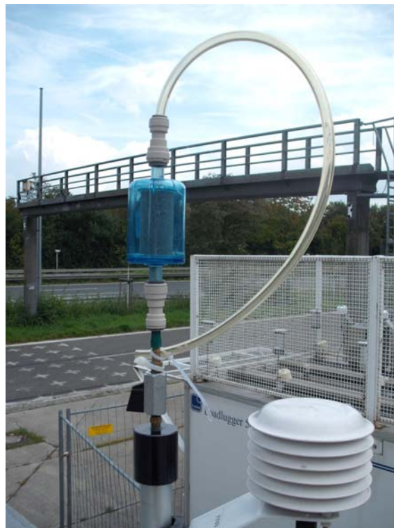
Figure 14: Zero-filter during field test
