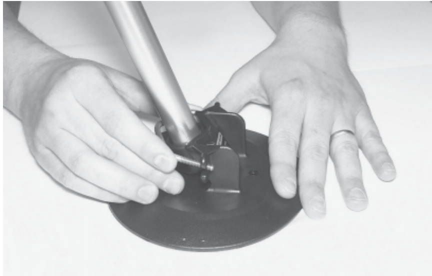
Figure 2-8. Placing the metal bracket on the tripod foot.
