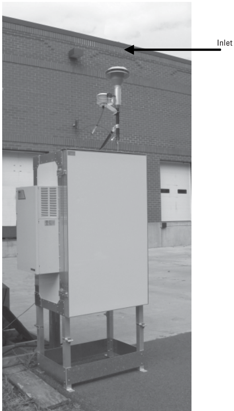
Figure 2-30. Outdoor enclosure with inlet installed.
