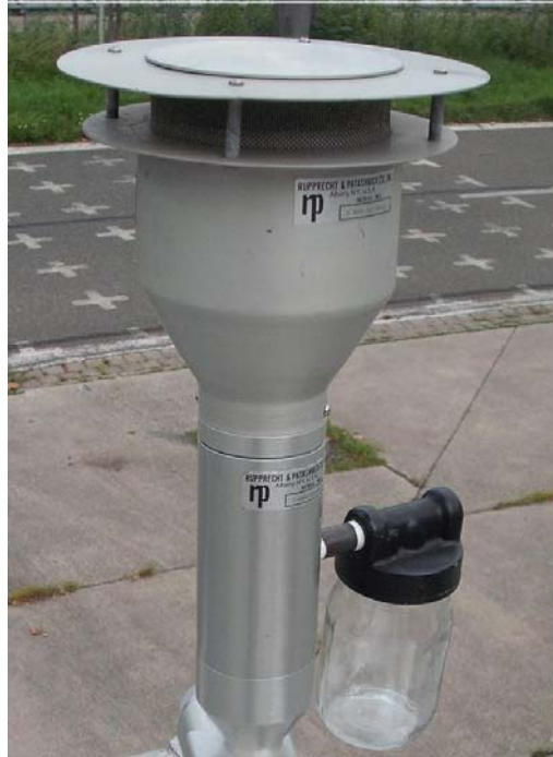
Figure 3: American PM 10 -sampling inlet (Original style, p/n 57-000596-0001) for TEOM 1405-F Ambient Particulate Monitor
