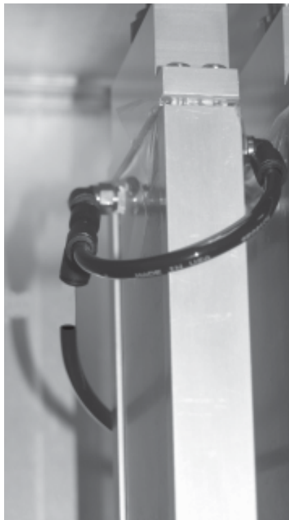
Figure 5-39. Main dryer vacuum line removed from T-fitting.
