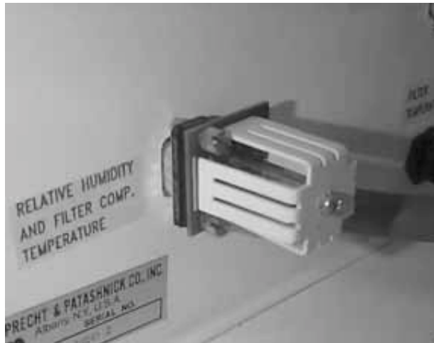
Figure 3-13. Relative Humidity and Filter Temperature Module
