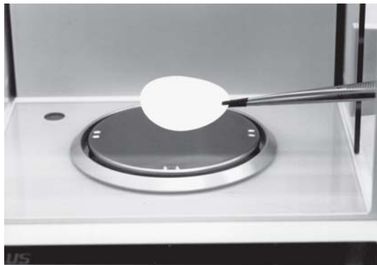
Figure 3–1. Positioning a 47 mm Filter on a Balance
