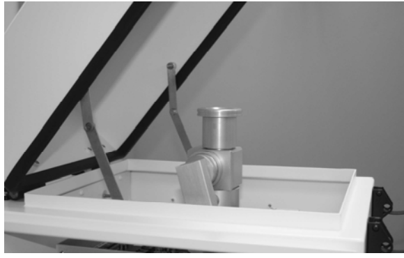
Figure 4-2. Sampler with VSCC Inlet Installed
