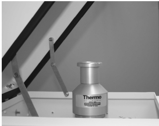
Figure 4-4. Sampler with PM 10 Inlet and WINS Impactor Installed
