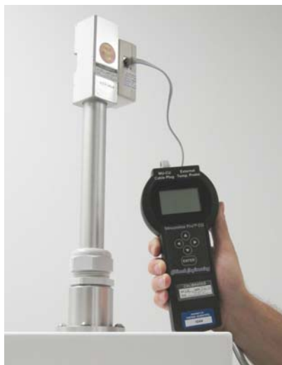
Figure 7–8. Streamline Pro Installed on External Sample Tube
