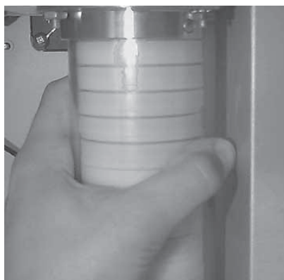
Figure 3–8. Rotating the Filter Cassette Magazine into its Locked Position
