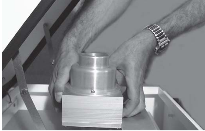
Figure 10–8. Removing the Virtual Impactor
