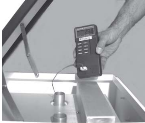
Figure 7-5. 2025i-D – Inserting an External Temperature Probe into the Rear Sampling Chamber
