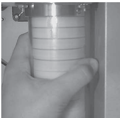
Figure 3–20. Reinstalling the Supply Filter Cassette Magazine into the Sampler
