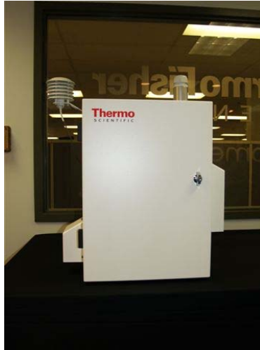
Figure 2–2. Sampler with a Large Rainhood Installed on the Right Side Panel of the Unit and a Small Rainhood on Left
