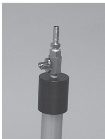
Figure 7–6. Flow Audit Adapter with Valve in Closed Position
