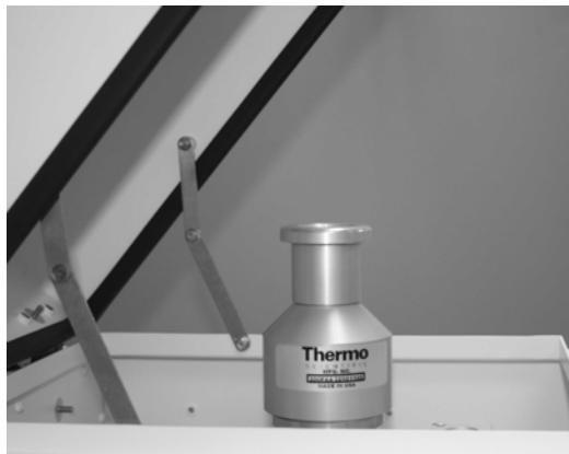
Figure 10–5. WINS Impactor in Upper Section of Enclosure
