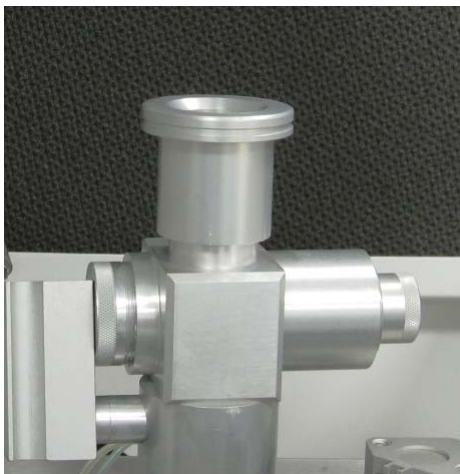
Figure 10–14. This Example Shows the VSCC Installed in the Sampler
