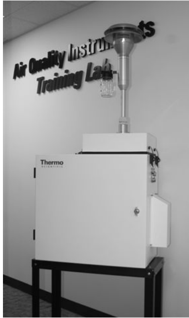
Figure 2–6. Sampler Mounted on Optional Stand
