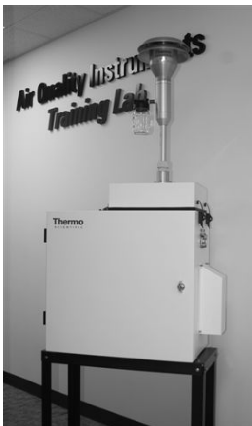
Figure 1–1. Partisol 2025 i and 2025 i -D Sequential Air Sampler
