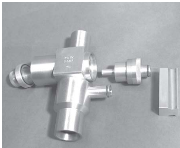
Figure 10–2. Main Components of the Cyclone Fractionator
