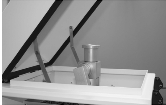
Figure 4-7. Open Top Cover to Access the WINS Impactor and WINS Adapter
