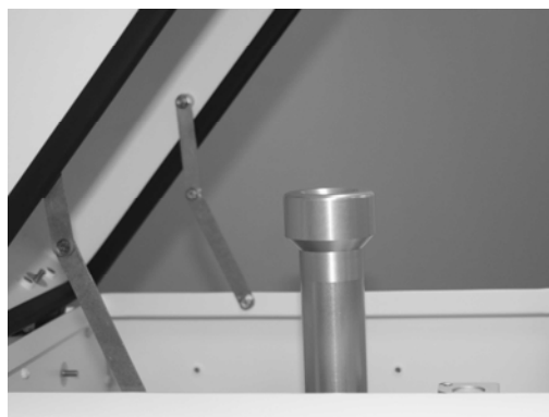
Figure 4–6. Sampler with Pass-Through Adapter Tube and PM 10 Inlet Installed
