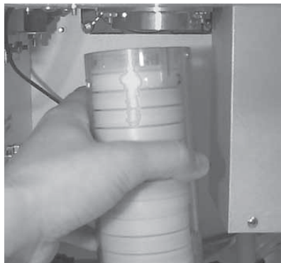
Figure 3–7. Positioning the Filter Cassette Magazine into its Mounting Location
