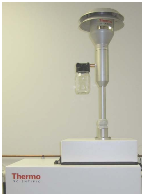
Figure 4–9. Installing the PM 10 Inlet
