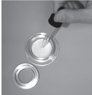
Figure 10–7. Coating the 37 mm Glass Filter with Oil
