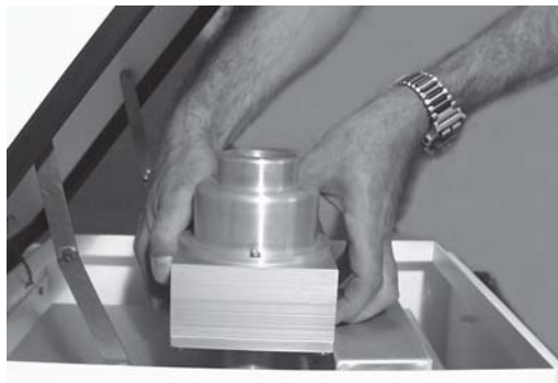
Figure 7-4. Removing the Virtual Impactor
