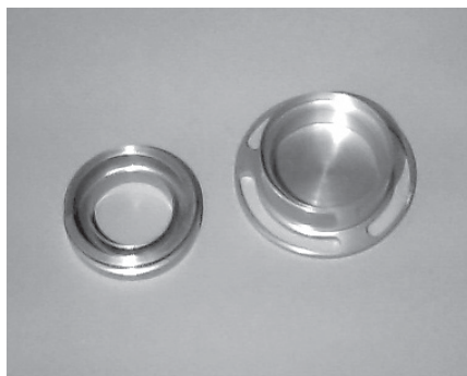
Figure 10–6. Upper and Lower Sections of the Impactor Assembly (on left and right sides of figure)
