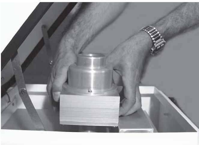
Figure 10–22. Removing the Virtual Impactor
