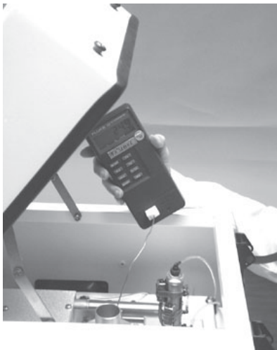
Figure 7-3. 2025 i – Inserting an External Temperature Probe into the Sampling Chamber
