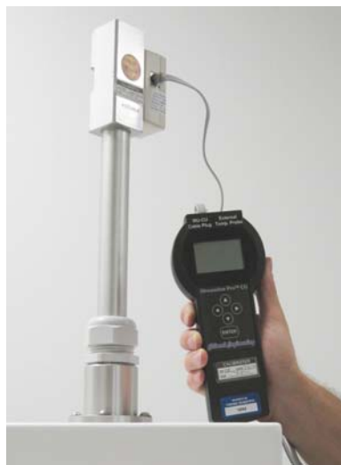
Figure 7-7. Streamline Pro Installed on External Sample Tube
