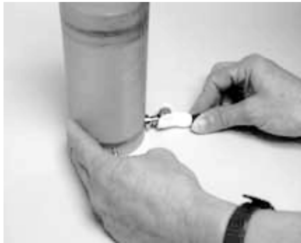
Figure 3-5. Attach bulb pump hose to magazine air connector.
