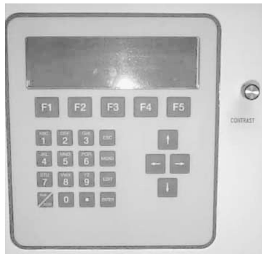
Figure 2-8. LCD contrast adjustment knob on right side of display/keypad.
