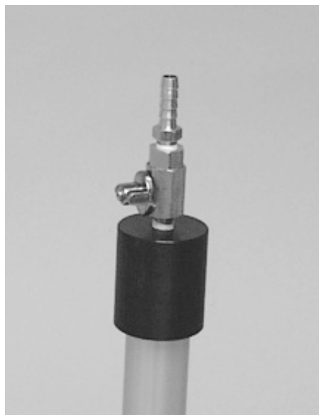
Figure 12-6. Flow audit adapter with valve in closed position .
