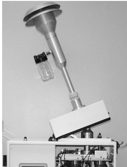
Figure H-12 (Right). PM-10 Partisol-Plus configuration.
