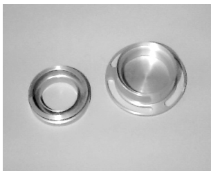
Figure G-6. Upper and lower sections of the impactor assembly (on left and right sides of figure).
