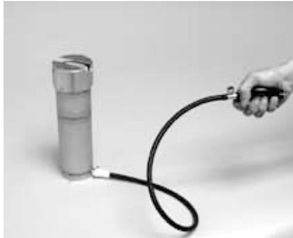
Figure 3-11. Squeeze gently on the bulb to push filter cassettes to the top of the cassette removal sleeve.
