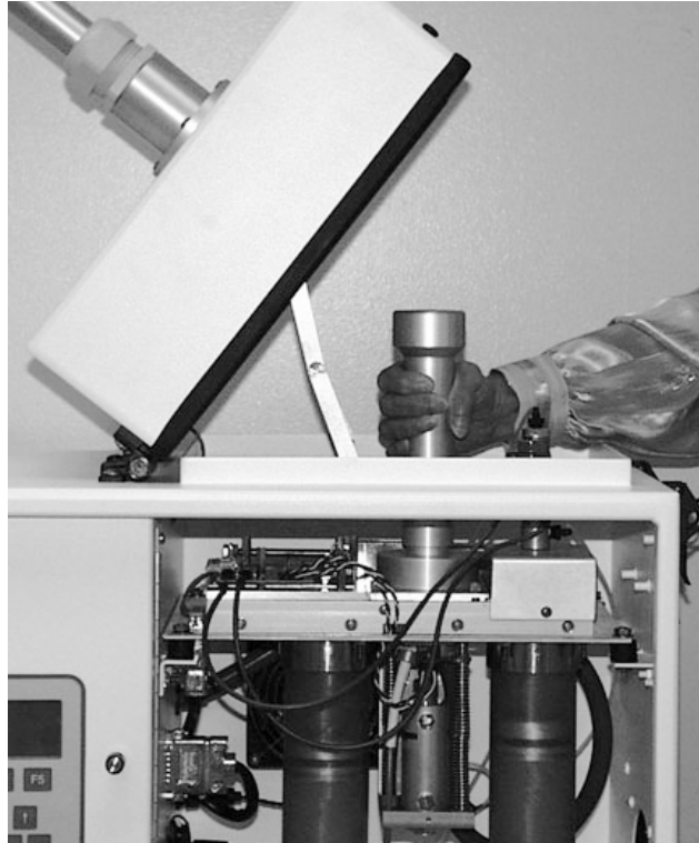
Figure H-8. Installation of the pass through adapter tube.
