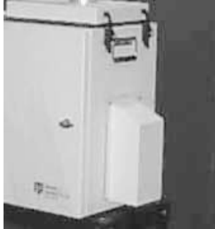
Figure 2-2 (Right). Partisol-Plus Sampler with two small rainhoods installed on the back panel of the unit.
