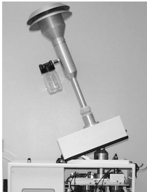
Figure H-2. Partisol-Plus Sampler with 1st stage inlet and WINS impactor installed.
