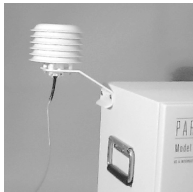
Figure 2-4 (Right). Ambient temperature probe plugged into the “ambient temperature” connector.
