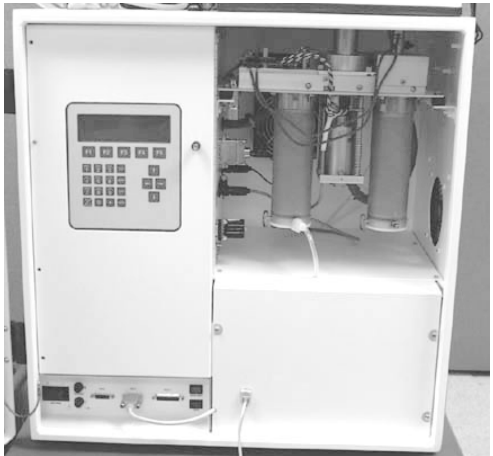
Figure J-6. Front view of a Partisol-Plus Sampler with an internal modem installed.
