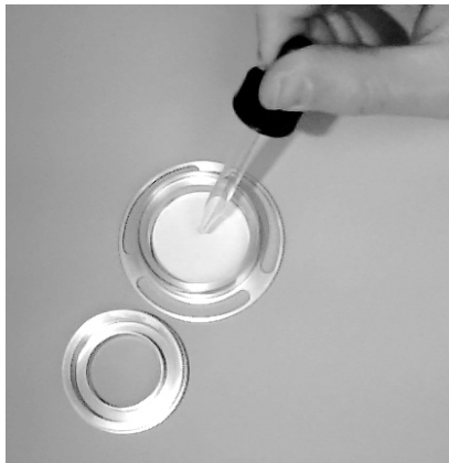
Figure G-7. Coating the 37 mm glass filter with oil.
