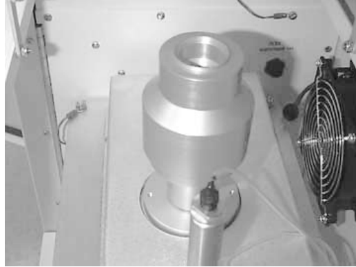
Figure G-4 (Left). WINS impactor in upper section of Partisol-Plus enclosure.
