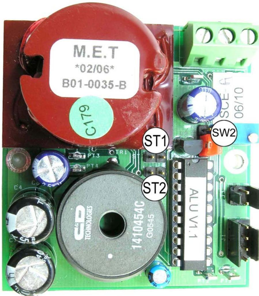
Figure 5-5 – Board of UV lamp, ozone generator option
