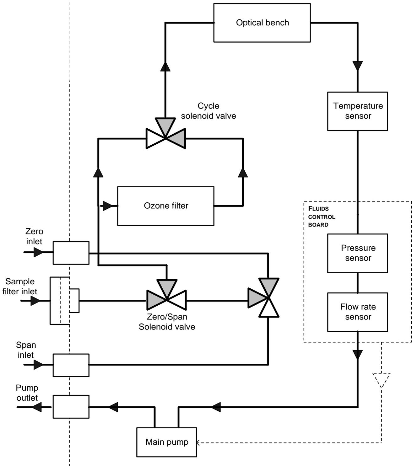
Figure 3-9 - Gas flow system with zero span solenoid valve
