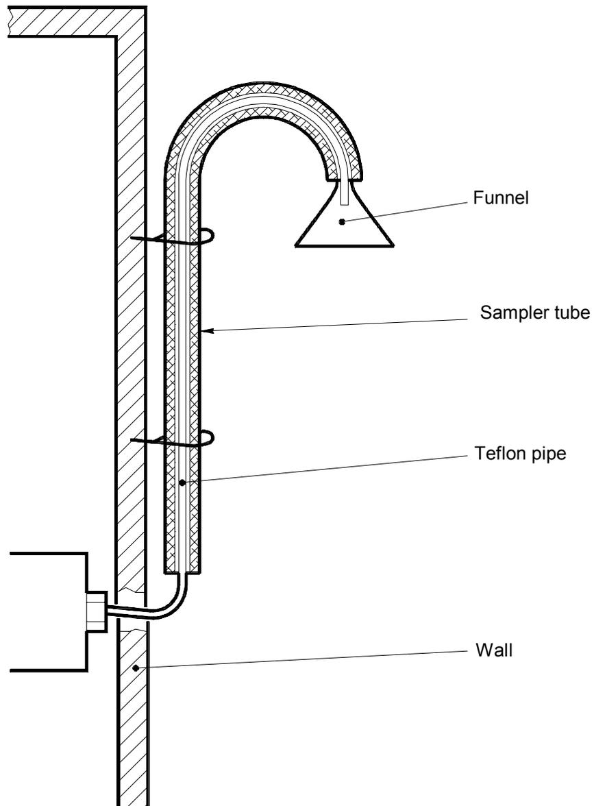
Figure 3-3 - Installation of the "sample gas" inlet
