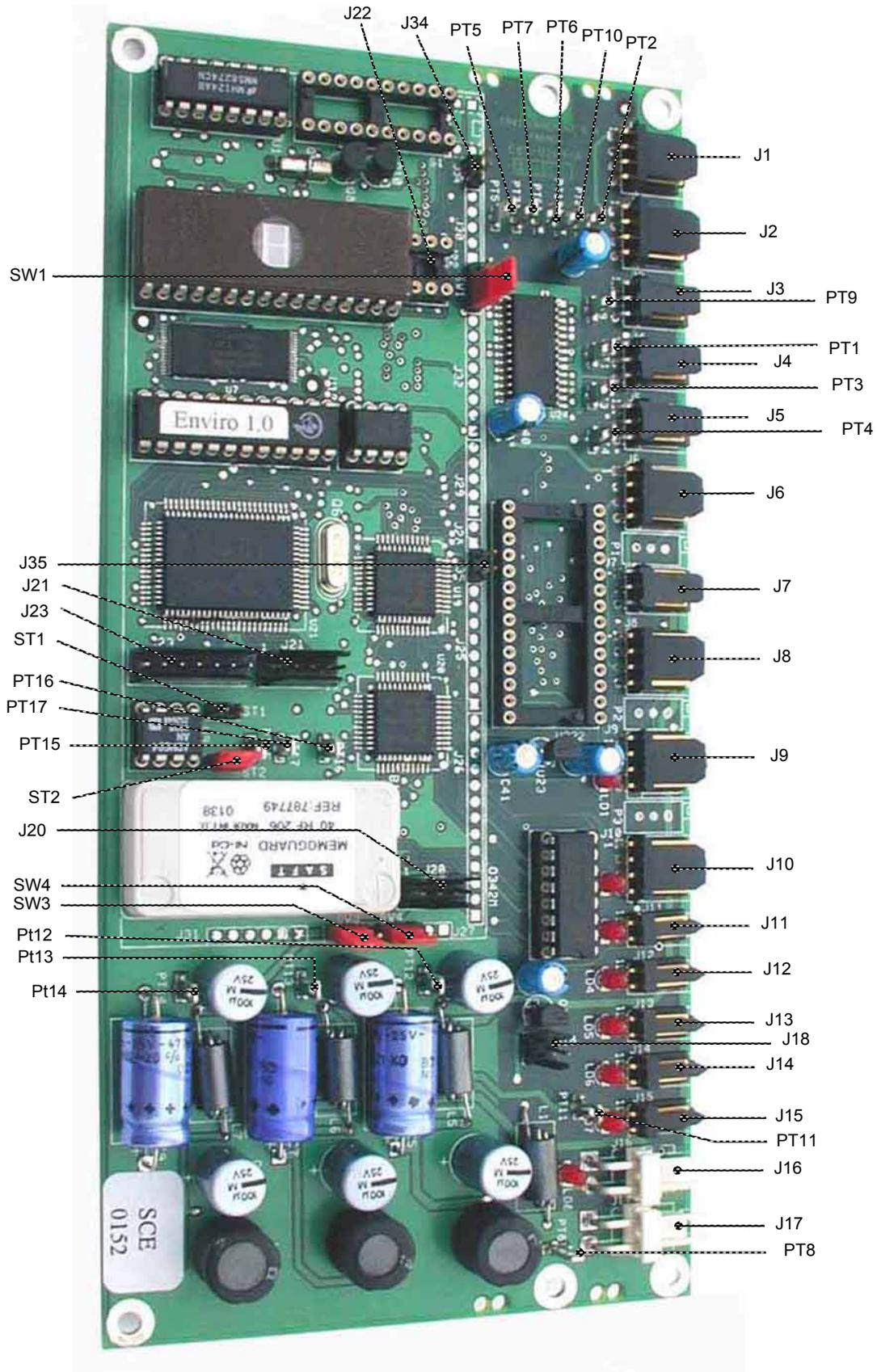
Figure 5-3 – MODULE board
