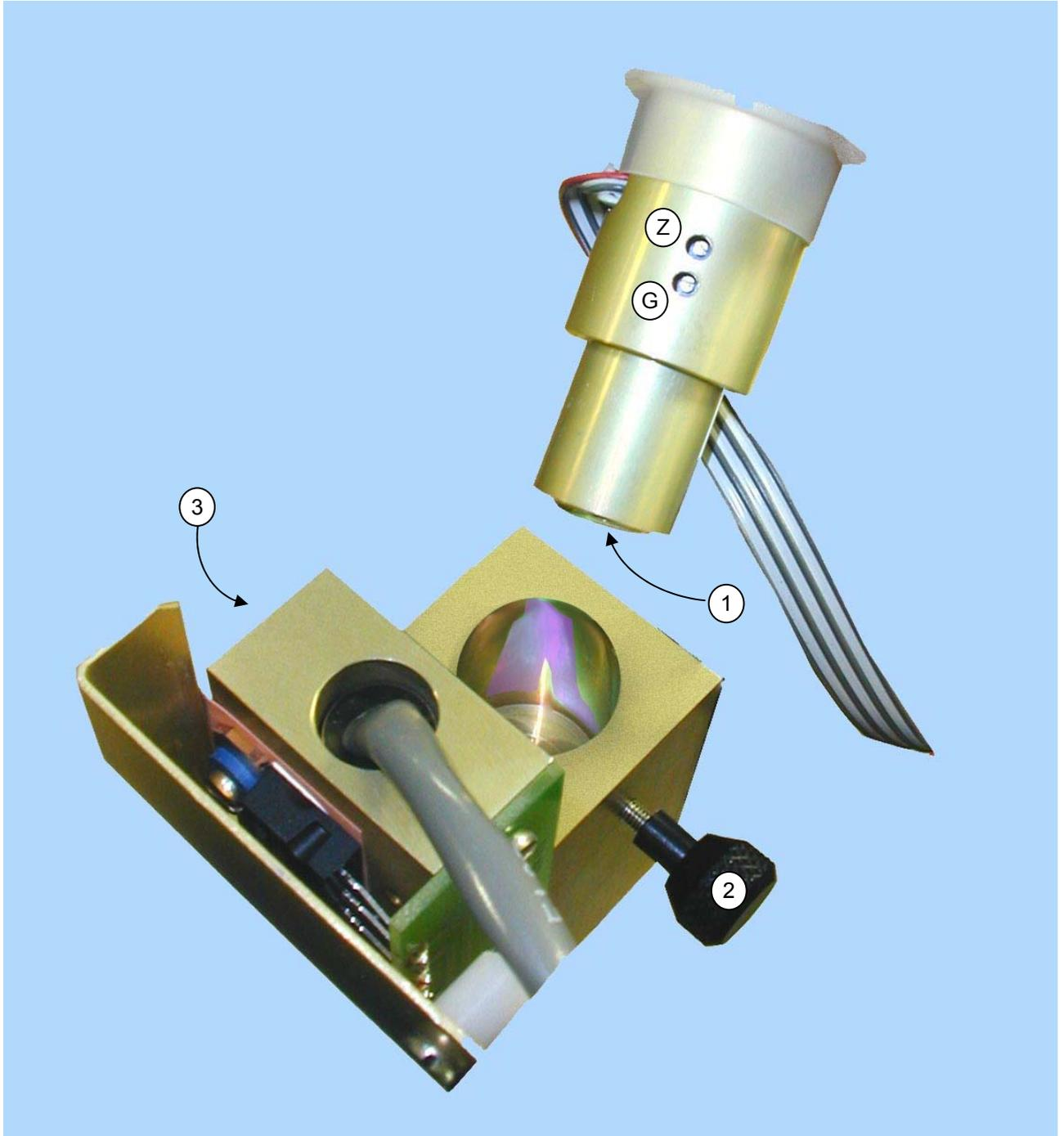
Figure 4-6 - Unlock and set detectors
