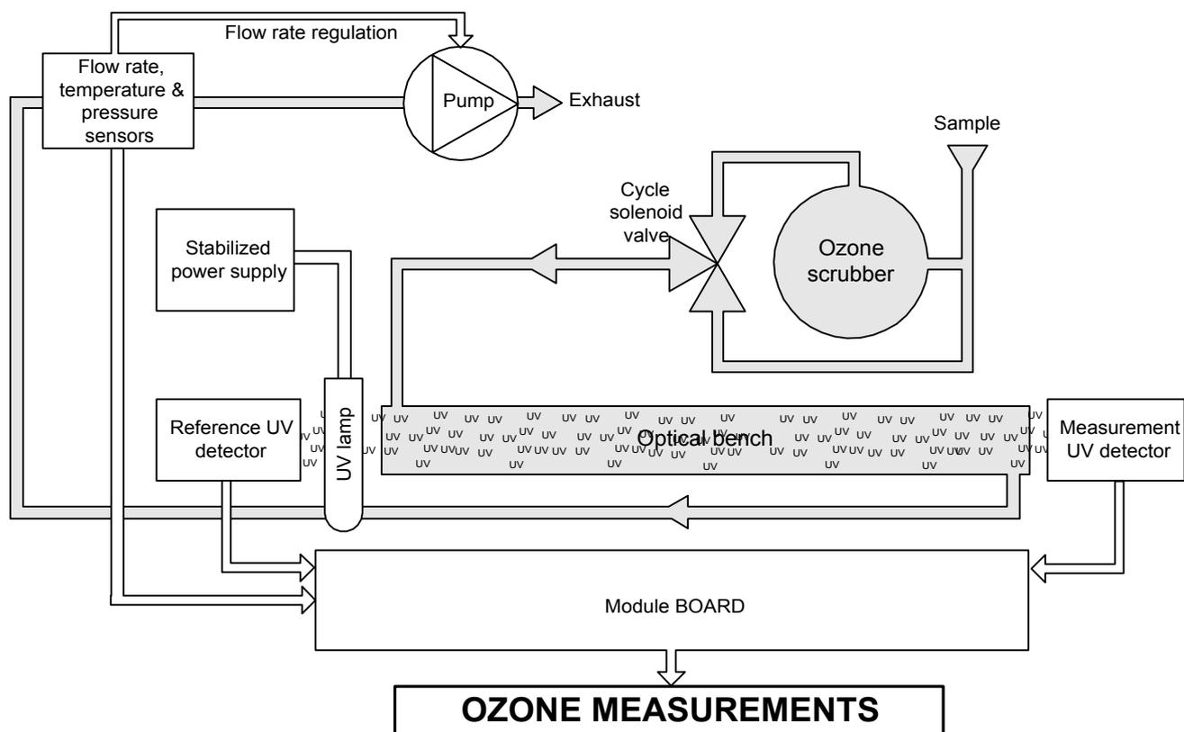
Figure 2-2 - General schematic diagram
