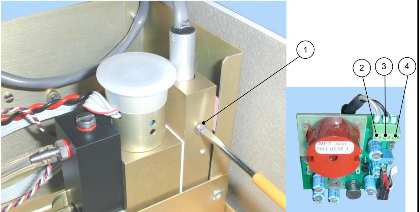
Figure 4-7 – Replacement of measurement UV lamp
