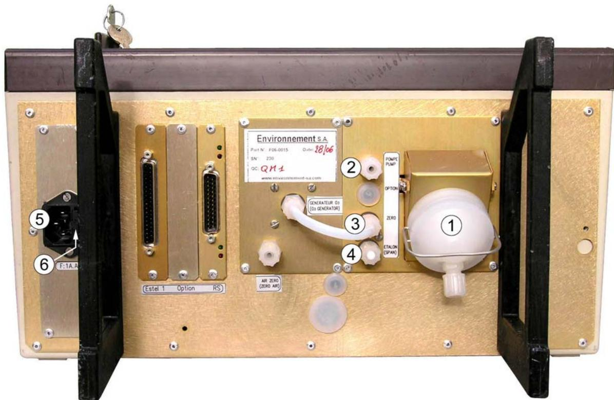
(1) dust filter, (2) pump outlet, (3) and (4) zero-span inlet, (5) electric connection plug, (6) fuse.
