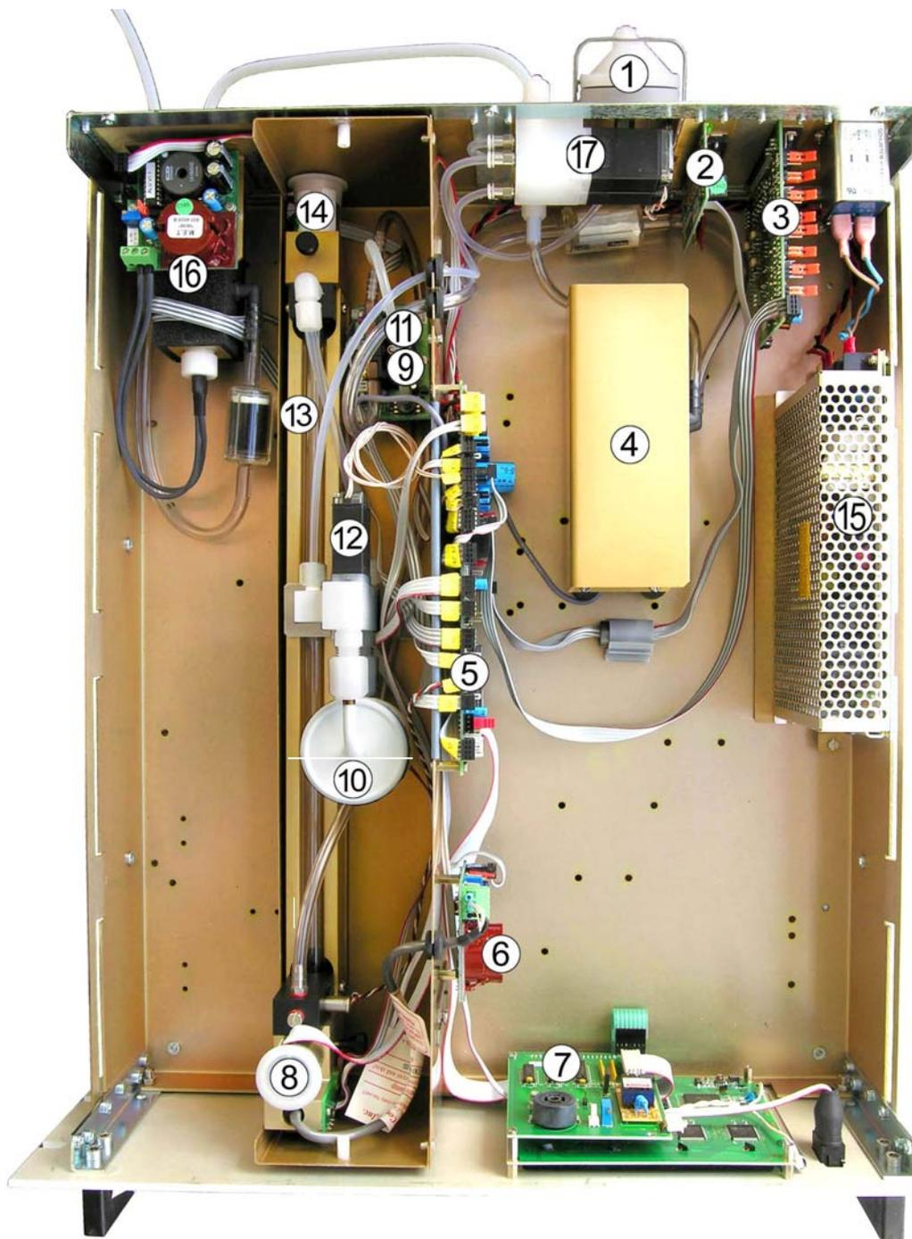
(1) dust filter, (2) RS232 series interface board, (3) inlet/outlet ESTEL board, (4) pump, (5) module board, (6) UV lamp supply, (7) interface board, (8) Reference detector, (9) barometre, (10) ozone purifier, (11) board of fluid checking, (12) 3-way solenoid valves, (13) measurement chamber, (14) Measurement detector, (15) 24V D.C. supply, (16) ozone generator, (17) Zero-Span SV block.
