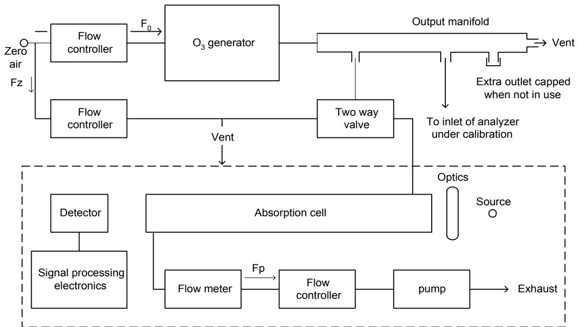
Figure 3-7 - Schematic diagram of a typical UV photometric calibration system (1)
