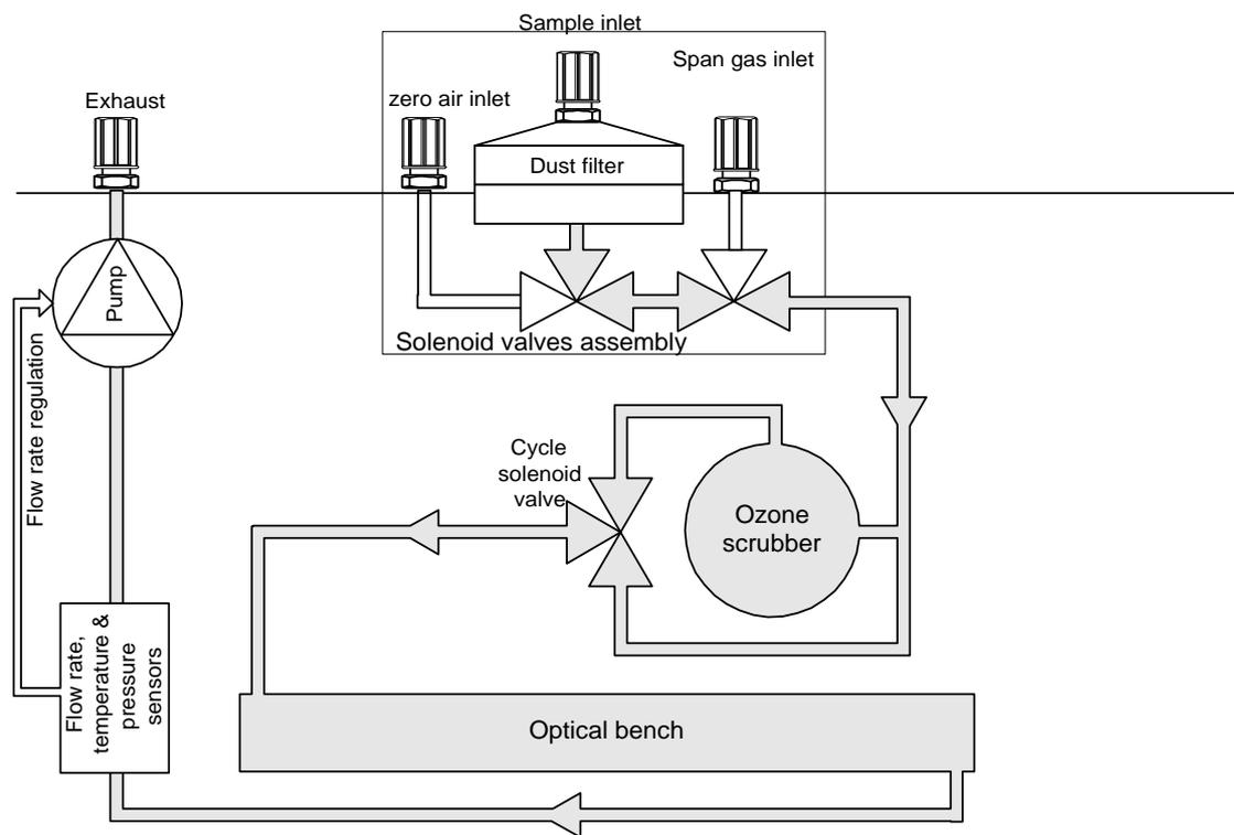
Figure 2-6 - Schematic diagram of gas flow system with solenoid valves option
