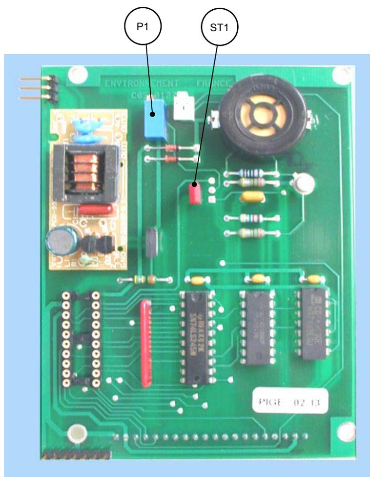
Figure 5-2 – Keyboard Interface board
