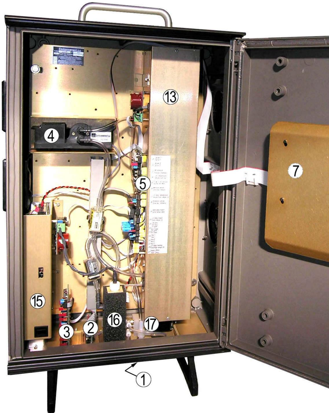
1) dust filter, (2) RS232 series interface board, (3) inlet/outlet ESTEL board, (4) pump, (5) module board, (7) interface board, (13) measurement chamber, (15) 24V D.C. supply, (16) ozone generator, (17) Zero-Span SV block.
