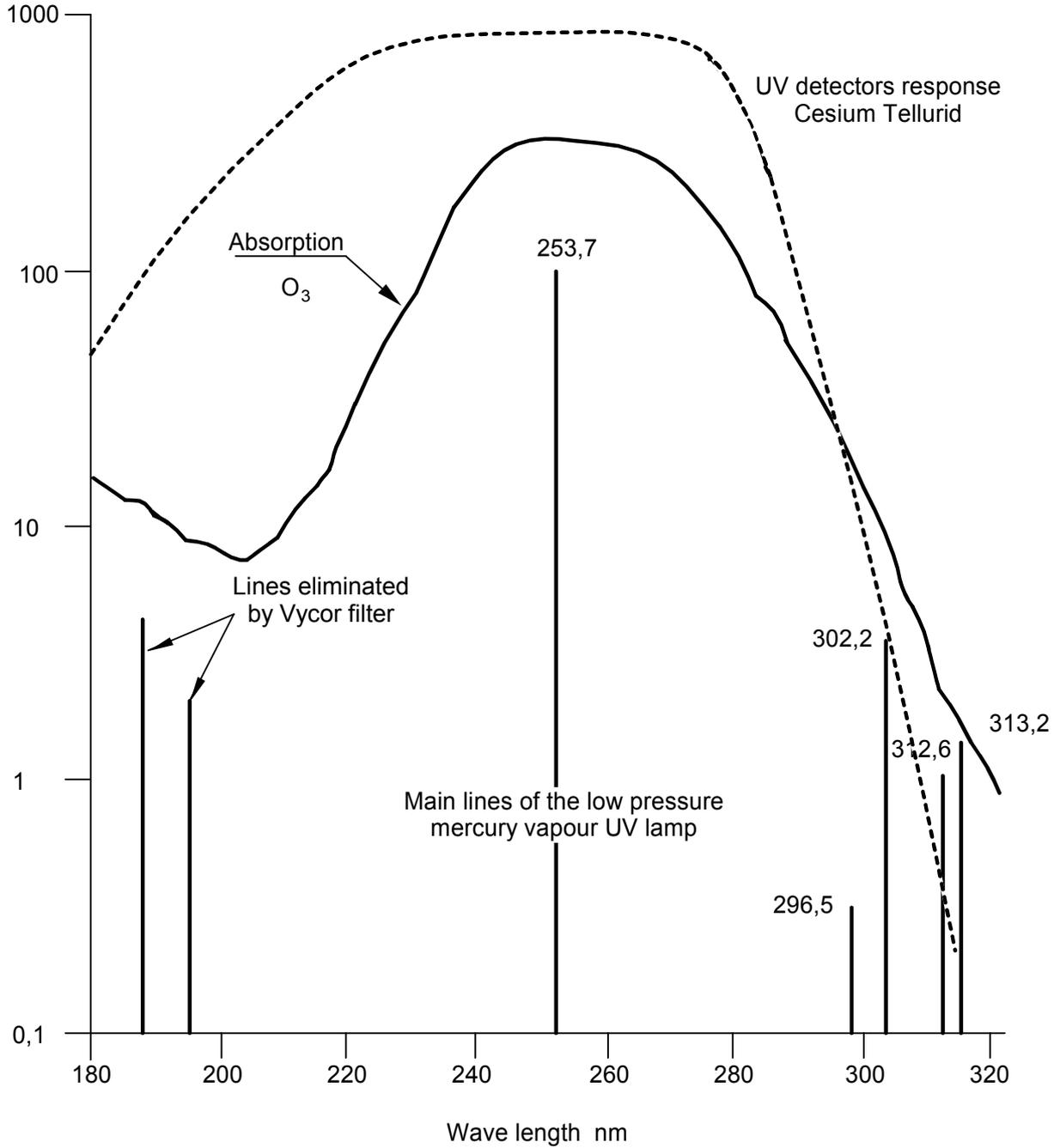
Figure 2-1 - Ozone absorption spectrum
