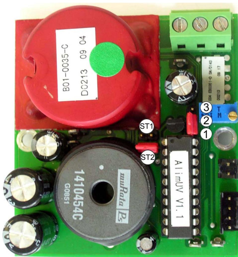
Figure 5-4 – Board of measurement UV lamp supply
