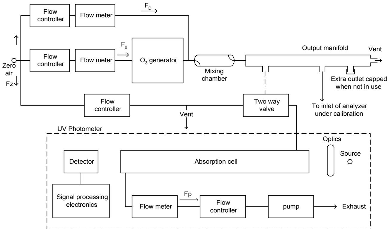
Figure 3-8 - Schematic diagram of a typical UV photometric calibration system (2)
