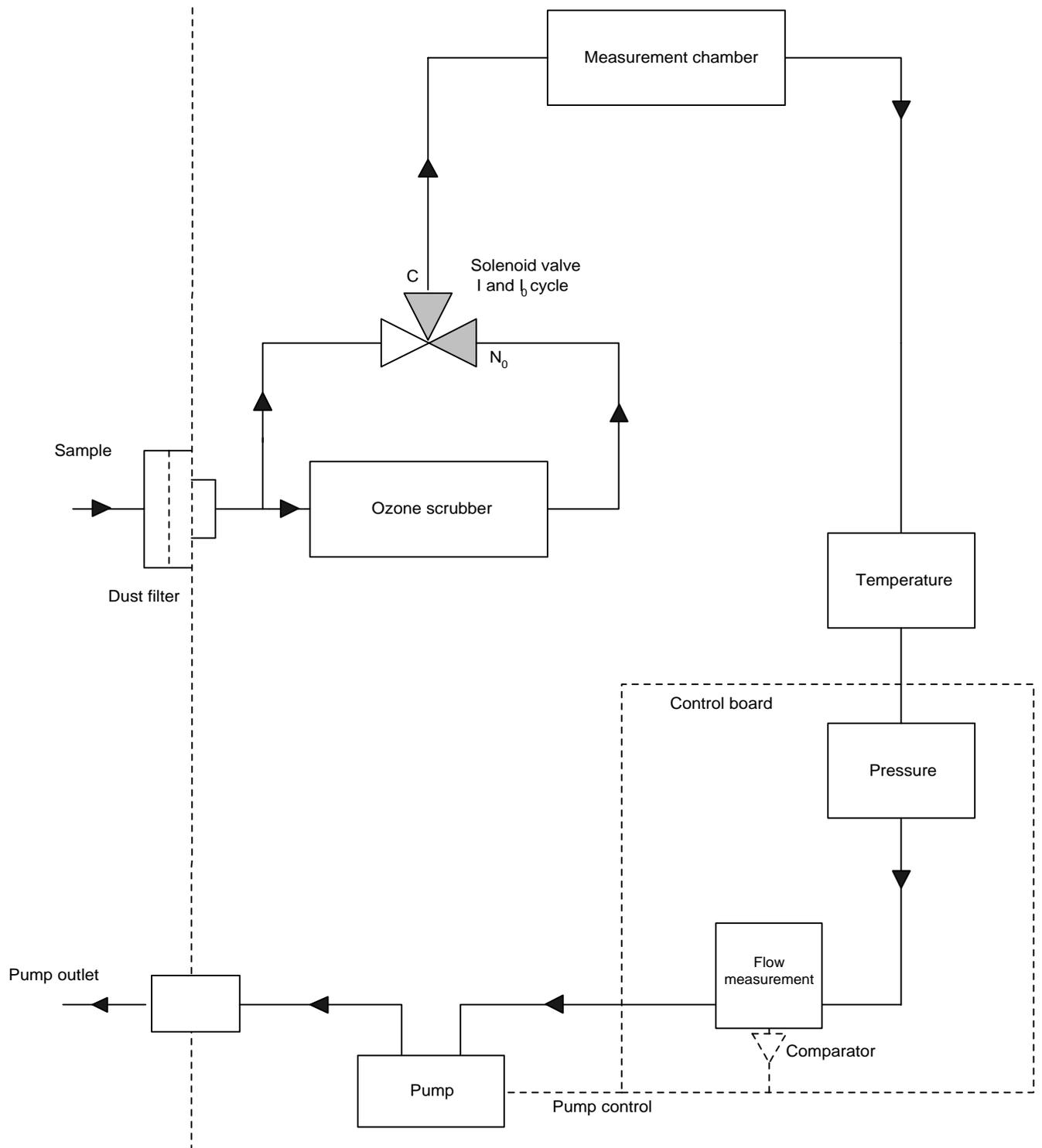
Figure 2-5 - Schematic diagram of basic gas flow system
