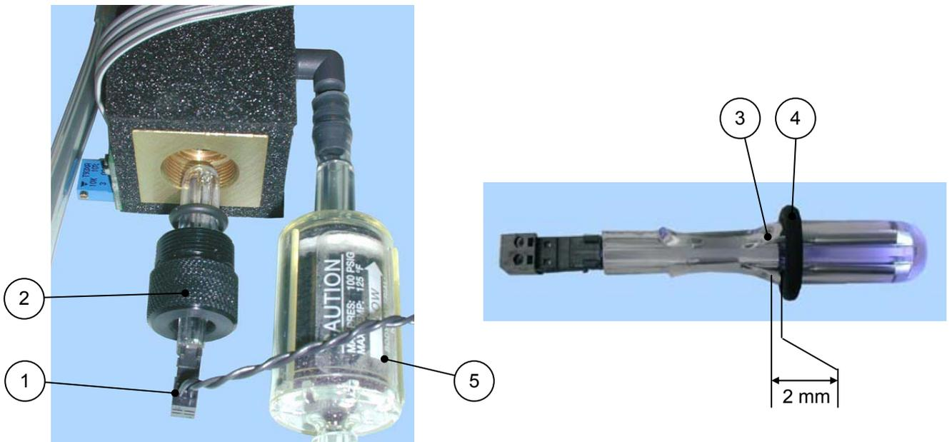
Figure 4-8 – Replacement of optional O<sub>3</sub> generator UV lamp
