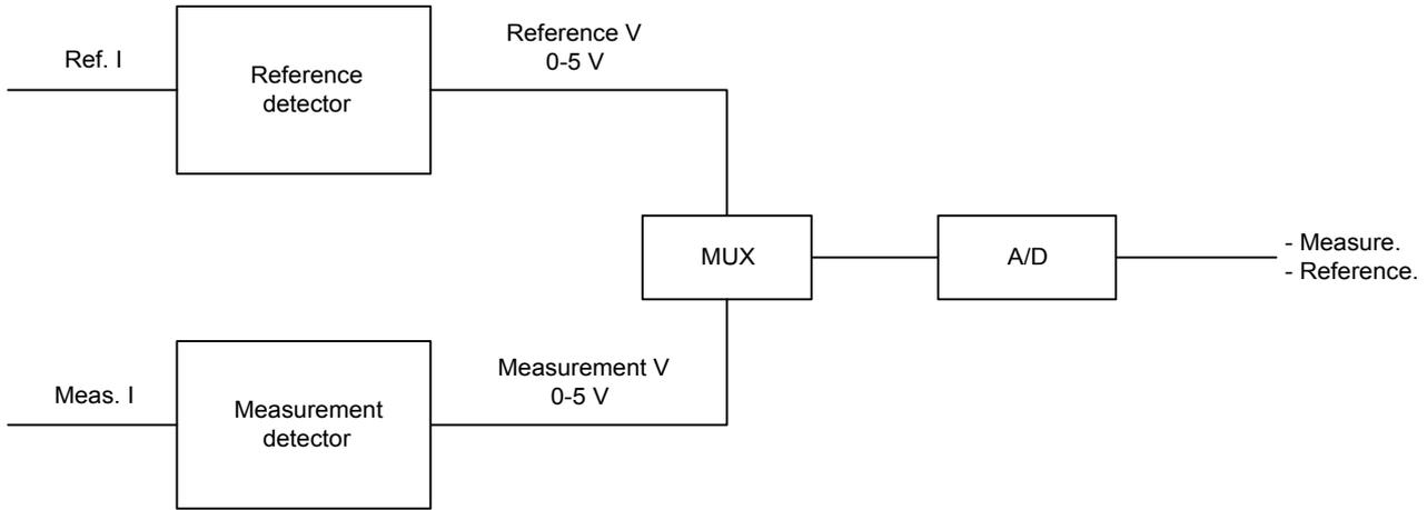
Figure 2-3 - Acquisition of UV energies I<sub>0</sub> and I
