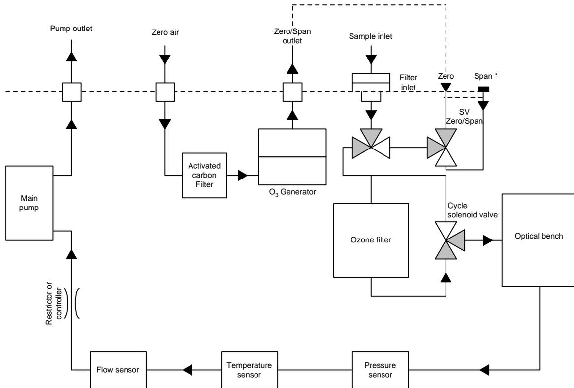
Figure 3-10 – Gas flow system with Ozone generator
