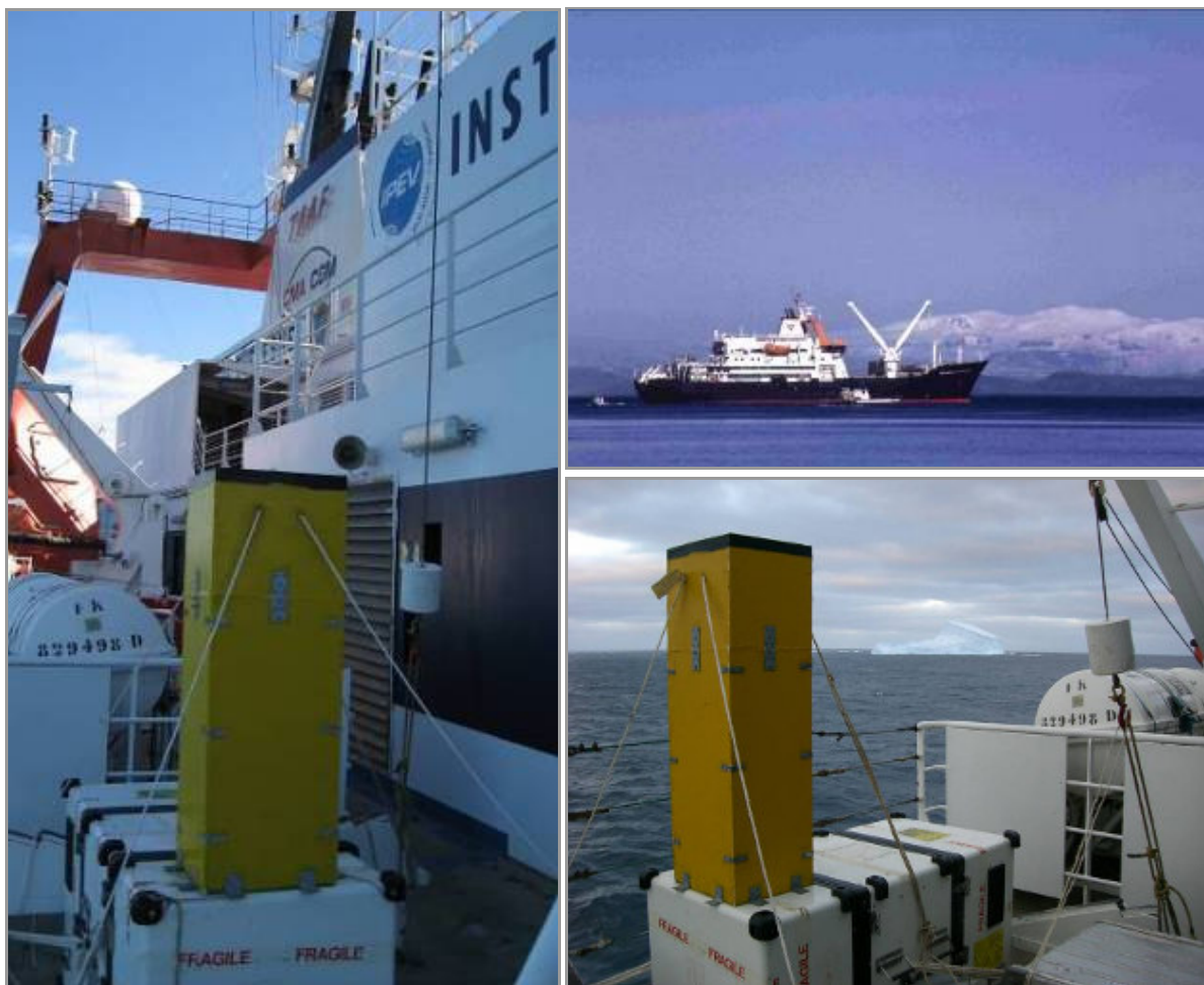
Figure 1 (left): EZ LIDAR ALS300 on board the “Marion Dufresne” oceanographic ship.
