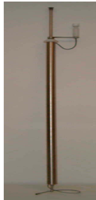
samplepipe 182 with attached temp./hum. sensor 1.153 FH 180 (delivered separately)
