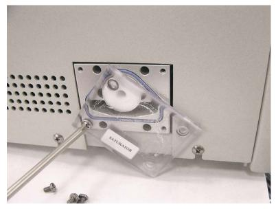
Figure 8-7 Saturator Wick Removal
