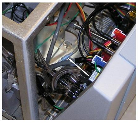
Figure 8-6 Micro-Pump Filter, Shown Behind the Opened Front Panel
