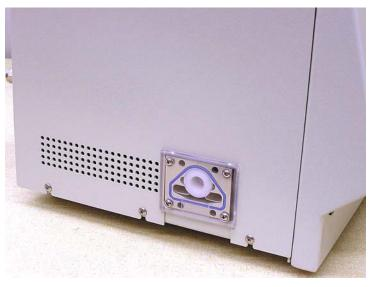
Figure 3-4 Left Side Panel Showing Butanol Reservoir and Saturator Wick
