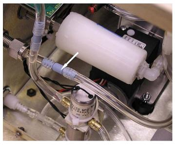
Figure 8-3 Replacing the Makeup Air Filter
