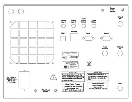
Figure 3-2 Back Panel of the Model 3775 CPC
