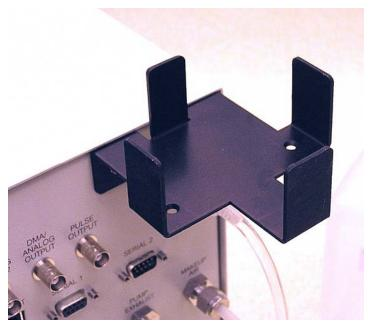
Figure 2-1 View of Fill Bottle Bracket Mounting
