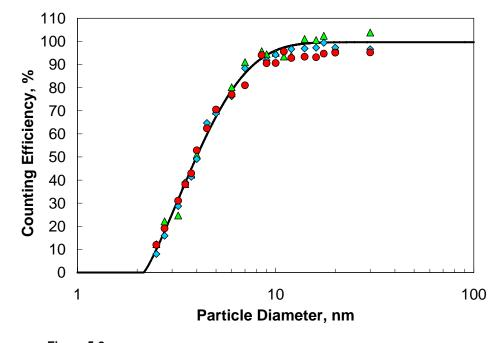
Figure 5-2 Counting Efficiency Curve of 3775 CPC
