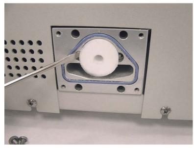
Figure 8-8 Prying the Saturator Wick Out
