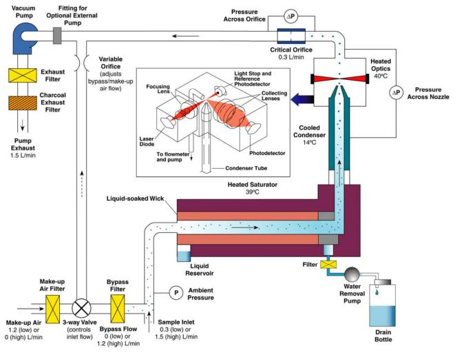
Figure 5-1 Flow Schematic of the Model 3775 CPC
