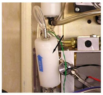
Figure 8-2 Replacing the Bypass Air Filter
