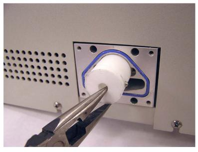
Figure 8-9 Pulling the Saturator Wick Out Using Pliers with Minimal Force
