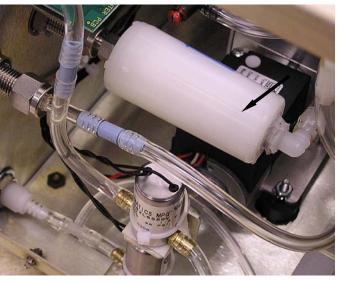
Figure 8-1 Replacing the Exhaust Filter
