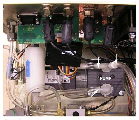
**Figure 8-12** Top View of Instrument Showing Pump Top and Pump Inlet and Exhaust Fittings and Tubing
