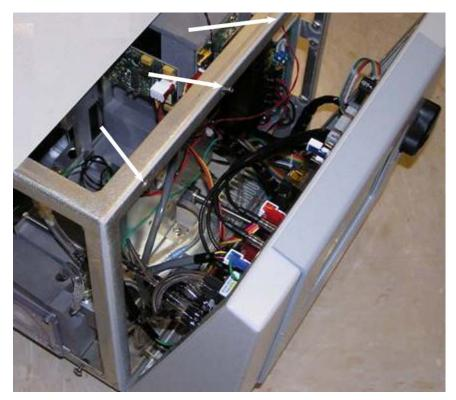
Figure 8-5 Front Panel Screw Removal
