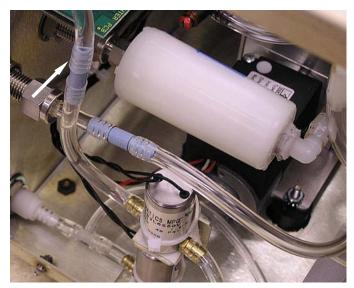
Figure 8-4 Replacing the Butanol Fill Filter
