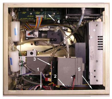
Figure 3-6 Electronics Boards Inside the Model 3775 CPC
