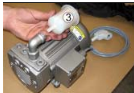
STEP 1 : remove the exhaust filter (3)
