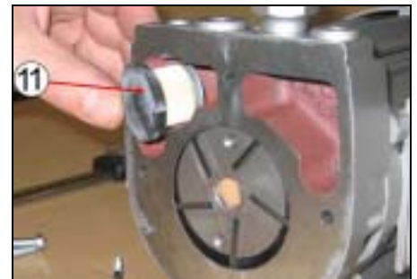
STEP 9 : reassemble the filter cartridge (11). Change it each time you do a vanes change.
