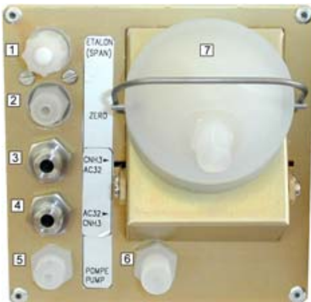
(1) span gas inlet – sealed in case of built-in permeation bench, (2) zero air inlet, (3) from NH 3 S 2 rack output, (4) to NH 3 S 2 rack input, (5) pump output, (6) zero air inlet of built-in permeation bench, (7) inlet of sample to be analyzed.
