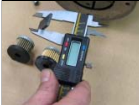
STEP 6 : check vane height. Change them if H < 11 \text{ mm}
