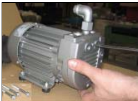
STEP 11 : screw on the flask (4 screws).
