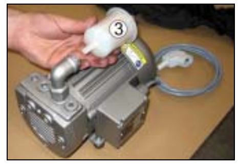
STEP 12 : Remount the exhaust filter (3). Change it on each vanes change.
