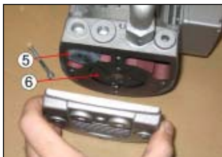
STEP 3 : remove the flask to have access to the filter cartridge (5) and the carbon vanes (6).
