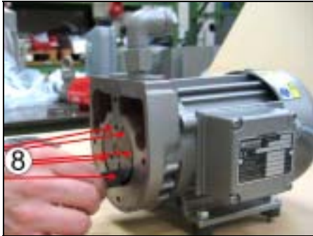
STEP 5 : remove the vanes (8). There are 5 vanes .
