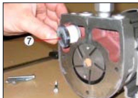
STEP 4 : remove the filter cartridge (7)
