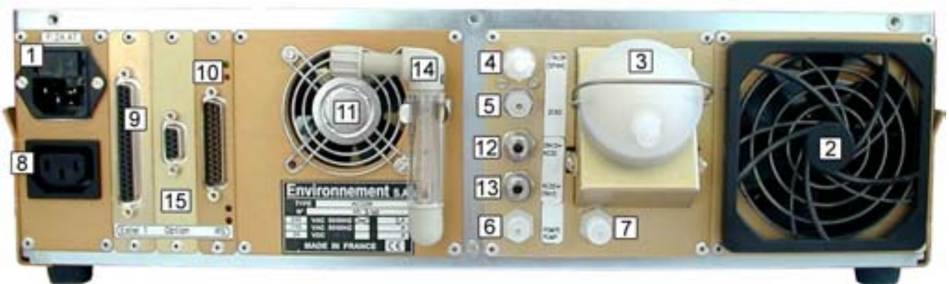
Figure 1-5 – Rear panel with permeation bench option and connection to CNH3 S2 rack
