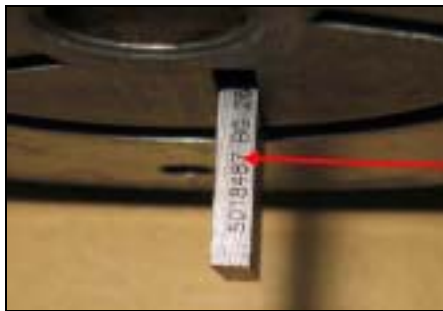
The marked side of the vanes must be upward oriented .
