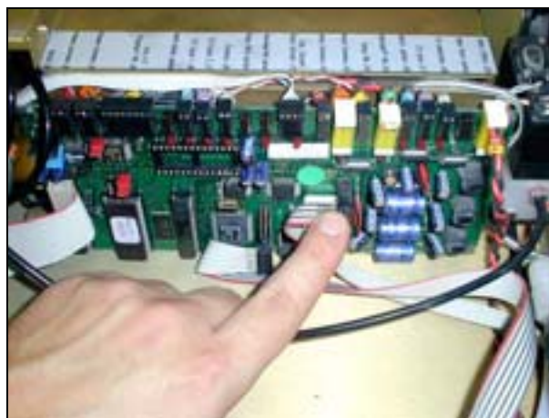
(4) Then, re-connect on Module board at J20
