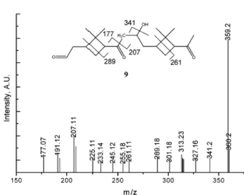
FIGURE 2. Product ion spectrum of the 359  $m/z$  precursor. Hydrogen rearrangements and/or dehydrogenation reactions that accompany many of these fragmentations are not shown in the inset.
