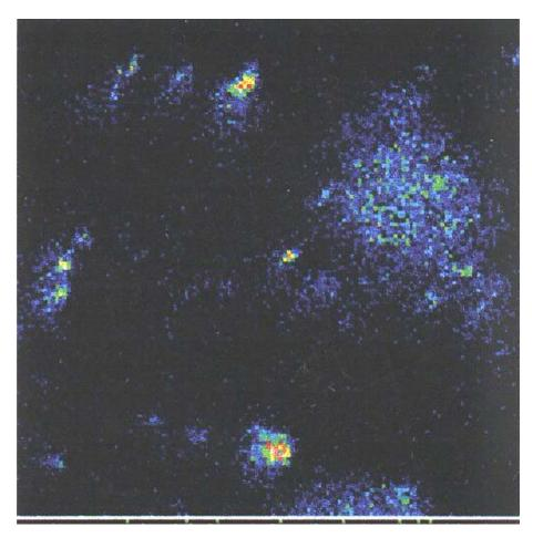
Figure 7. SIMS image of some  $SiO_2$  particles,  $Si^+$  spatial distribution. When particles are collected on the substrates, they can be found by COSIMA's primary ion source looking for indicative mass lines. Here is an example for silicate particles, detected by the  $Si^+$ -intensity-distribution.
