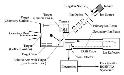
Figure 1. Schematic view of the COSIMA instrument: (1) Dust is collected on metal targets, (2) Positions of dust grains are determined by microscopic camera, (3) A pulsed primary ion beam sputters and partially ionizes the cometary material, (4) Secondary ions are accelerated by an electric field and travel through the time-of-flight section – a drift tube with an ion reflector, (5) Mass spectra data are extracted from the resulting time-of-flight spectra.
