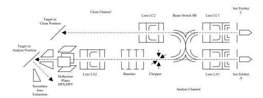
Figure 10. Schematic sketch of the Primary Ion Beam Subsystem design: Ions from two emitters at the right side can reach either of two positions: 'Analyze' or 'Clean', depending of the 'Beam Switch' in the center. The focusing elements are electrically shared, as only one beam can be active at any time. 'Chopper' and 'Bunchers' provide the pulsed beam for analysis, the deflection plates are used for steering the beam spot on the target.
