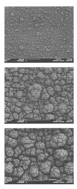
Figure 6. SEM picture of a liquid-deposited black. These collection substrates are thicker than those made by vapor deposition, and can be made from different materials. They usually show a 'cauliflower' like surface structure, in which smaller grains could be trapped and escape analysis.
