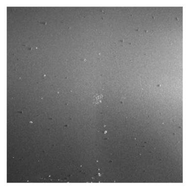
Figure 8. COSISCOPE image of a  $2 \times 2 \text{ mm}^2$  region on a collector substrate exposed to silicate dust. The low incidence light comes from the right. A cluster of silicate particles is visible in the center. Other dark 'low velocity' grains stick on the surface with long shadows extending to the left. The bright spots are scratches or blank metal particles from the (early) production process. The noise level from the substrate is acceptable even under shallow illumination.
