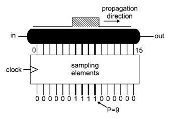
Figure 16. Time-to-position principle. The pulse from the detector amplifier moves from left to right through the delay line and, at a given time, is detected by several elements. The '1's are later interpreted by the software to derive the exact time of the event.
