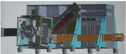
Figure 2. COSIMA instrument (flight model and 3D drawing). The COSIMA flight model consists of dust funnel, target manipulation unit (TMU), primary indium ion sources (PIS) with the primary ion beam subsystem (PIBS), the high-resolution mass spectrometer with ion detector, all mounted onto the COSIMA electronic box.
