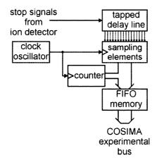
Figure 15. TDC Block diagram of the COSIMA time-to-digital Converter: The data from the tapped delay line and the master clock counter are added and stored in a hardware device until the instrument's processor can pick up the data.
